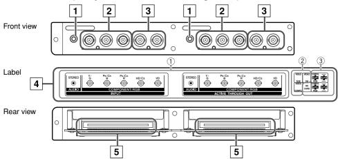
1 Audio signal input (INPUT)/output (ACTIVE THROUGH OUT) terminals Accepts/outputs analog audio signals.
